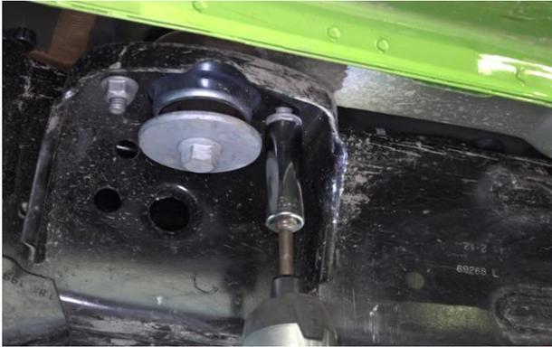
**NOTE:** If you choose to install the optional hardware, proceed to step 5) prior to fully installing all hardware. Tighten a few nuts to hold the slider in place while marking the hole location.
