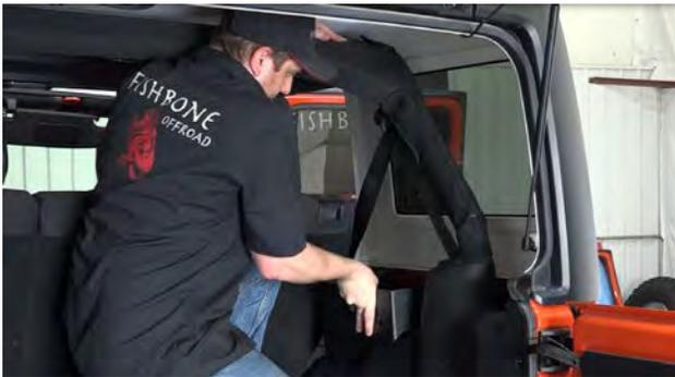
Either using all of your OEM hardware, or the supplied four (4) knobs and washers, secure the storage bins in place. Reuse your factory hardware to finish securing your hard top.
