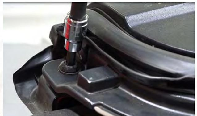
Remove the remaining six (6) torx bolts (3 on each side) from either side of the hard top from inside the Jeep.
