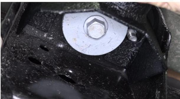
Remove the step slider and drill the marked location with a 7/16" drill bit. Use a smaller drill bit and step up in size if necessary. A centerpunch is also recommended to aid in starting the hole.
