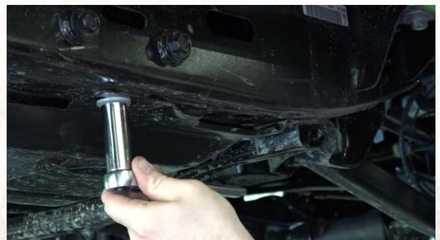
Remove the nuts from the rear-most body mount using a 16mm socket. For 4DR models, repeat this step on the middle body mount.
