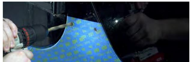
Remove the tape from around the holes, if necessary. This will prevent the tape from being caught behind the nutserts.
