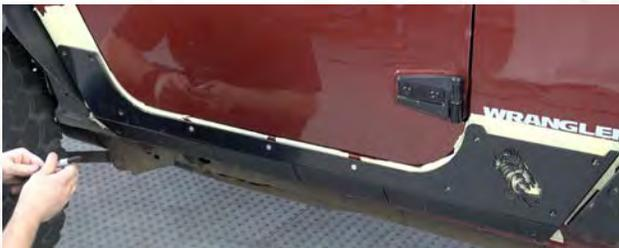
With the part on or off, carefully centerpunch or predrill the hole locations.
